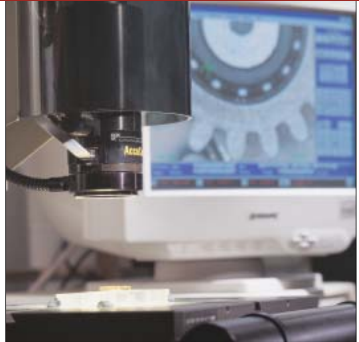
A vision system quickly verifies print conformance.
